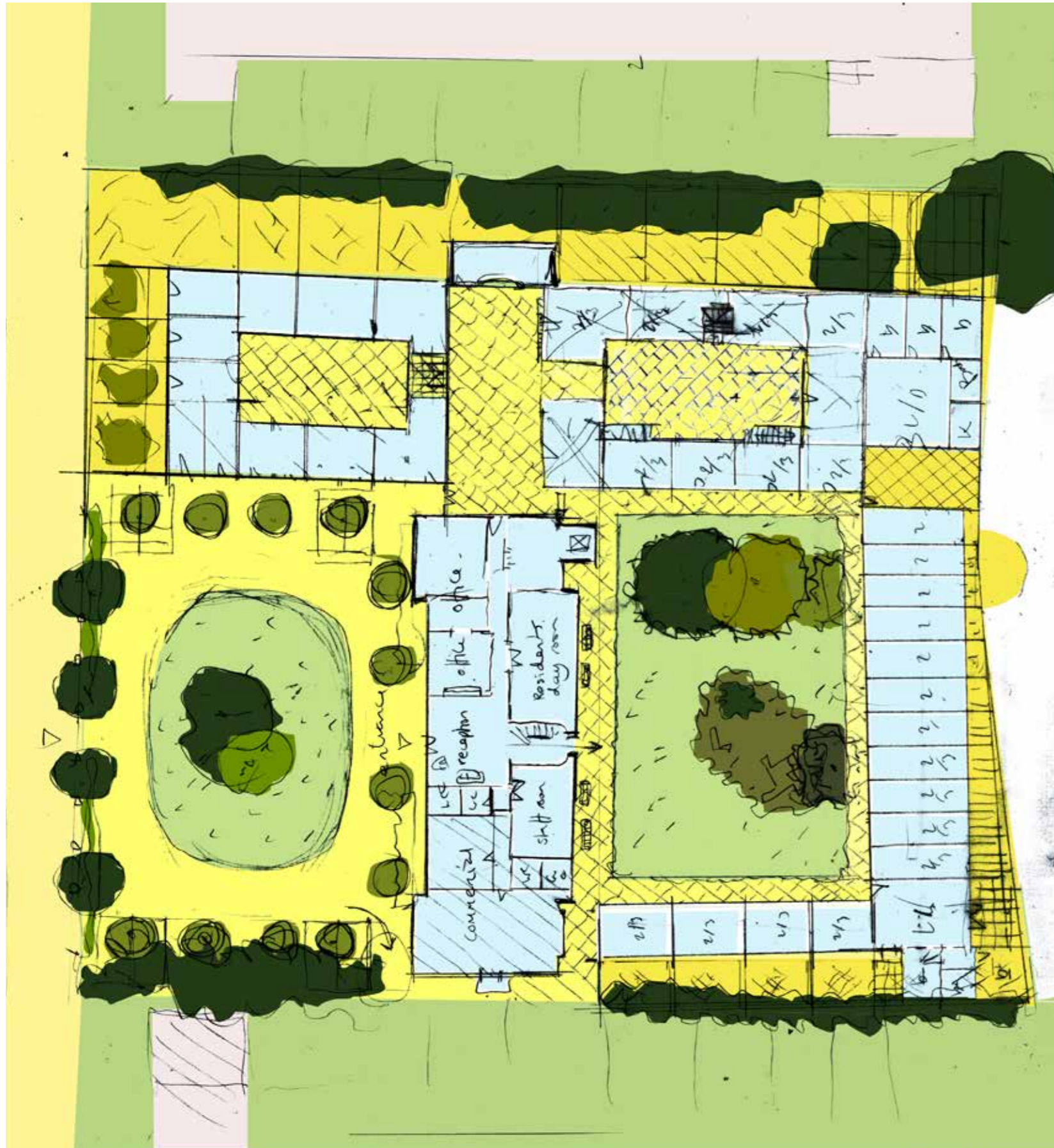
Plan sketch showing the proposed arrangement of new build accommodation around a series of courtyards and a communal garden
